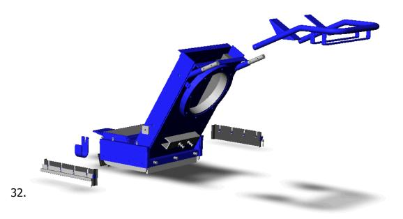
The machine will now fit through a 24"-man hole. Before building up the machine clean the body and the blastwheel with air. Inspect the body, seals and brushes. Replace them when they are damaged or worn.
